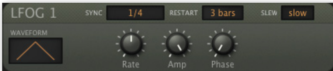
LFOG module, sine wave, synced to 'beats' and retriggered every 3 bars
