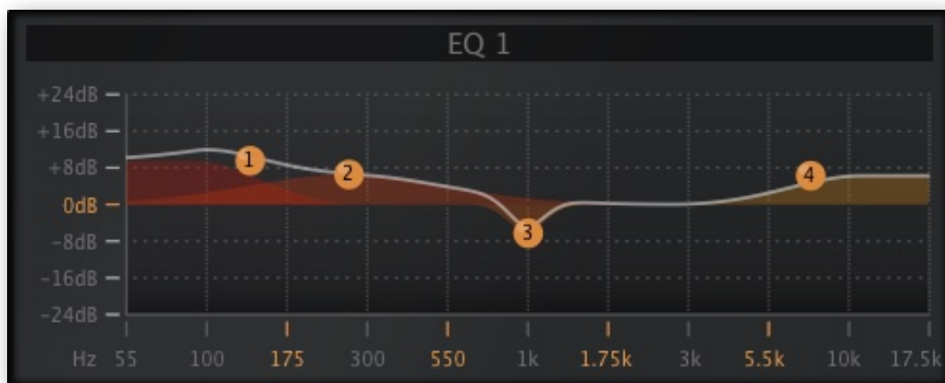
Equalizer module, bass+treble boost, dip around 1 kHz
