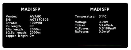
The Pulse16 MX shows the parameters of the SFP module installed. This can be helpful in troubleshooting or bugfixing.
