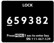
After entering the correct PIN, keep the MENU button pressed for one second. The device is locked now. Follow the same procedure to unlock the device again.
