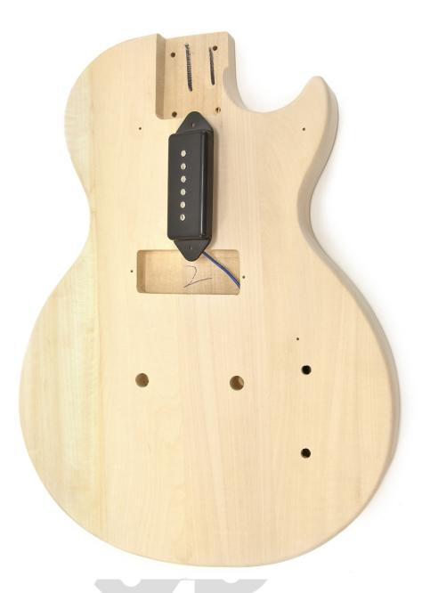
Feed the wire from the Pickup (3) through the hole into the body (1) cavity as shown in the picture, and then screw the Pickup (3) into place using the 2 x 18mm screws.
