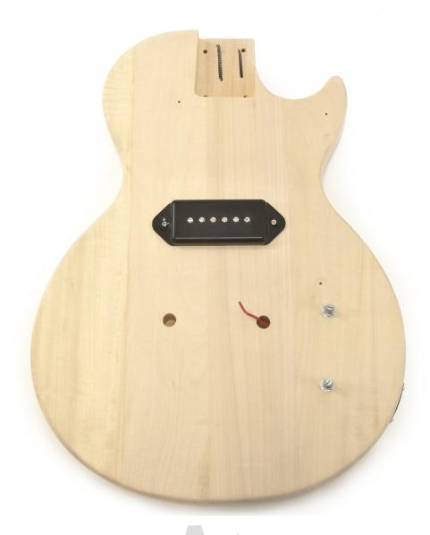
Solder the Earth Wire that has previously been thread through the body to one of the Bridge Pins (8), and insert the second Bridge Pin.
