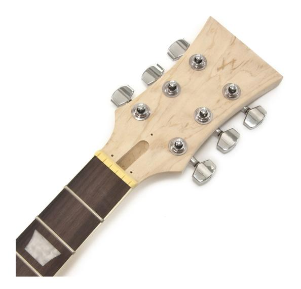
Insert the machine heads (10) in to the holes in the Headstock (2). Place the washer (11) on top, and then screw in the Ferrules (12). The neck should then be turned over and the 6 x 5mm screws should be screwed in to the pilot holes securing the machine heads in place. Make sure that the screw hole in the Machine Heads are facing downwards.
