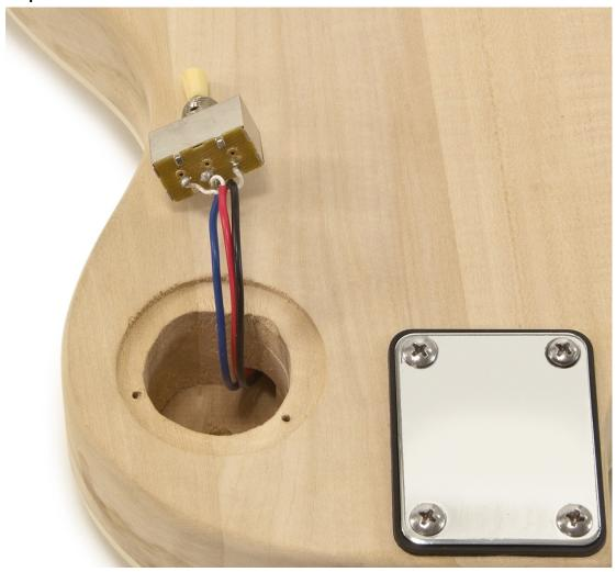
Pull the conjoined wires from the pre-wired circuit out of the tone selector cavity. Solder the coupled uncovered wires to the body arm on the back of the Tone Selector (5). Solder the covered output wire (Red) to the central middle arm of the Tone Selector. Solder the covered wire of the Neck Pickup (Blue) to the left central arm of the Tone Selector. Solder the covered wire of the Bridge Pickup (Black) to the right central arm of the Tone Selector.
