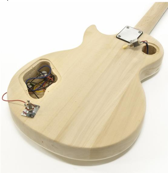
Solder the covered output wire to the long arm of the Jack Input (8). The uncovered wire should be soldered to the shorter arm. Solder the covered wire of the Neck Pickup (3) on to the middle arm of the first pot on the pre wired wiring (the pot without the transformer). Solder the uncovered wire on to the back of the first pot. Repeat this with the Bridge Pickup (4) and the second pot. Please refer to the wiring diagram for further explanation of this.
