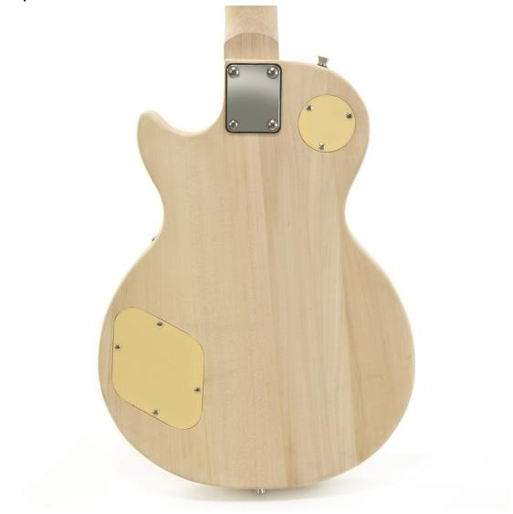
Put the Body (1) and Neck (2) together. Place the Neck Plate (14) with the rubber Pad on the back of the Body (1) in line with the pilot holes, and attach with the  $4 \times 45$ mm screws.
