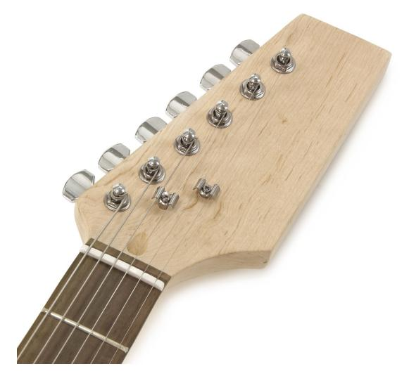
Insert the machine heads (16) in to the holes in the Headstock (2). Place the washer on top (18), and then screw in the Ferrules (17). The neck should then be turned over and the  $6 \times 10$ mm screws should be screwed in to the pilot holes securing the machine heads in place.
