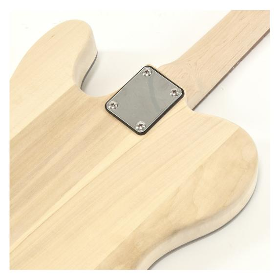
Put the Body (1) and Neck (2) together. Place the Neck Plate (19) with the rubber Pad on the back of the Body (1) in line with the pilot holes, and attach with the  $4 \times 45$ mm screws.
