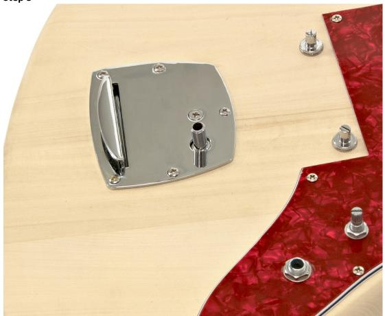
Screw the Tailpiece (13) in place, aligning it with the pilot holes, using the  $7 \times 25$ mm screws. Put the Bridge Pins (14) in the holes as pictured.
