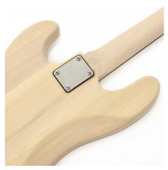
Put the Body (1) and Neck (2) together. Place the Neck Plate (5) with the rubber Pad on the back of the Body (1) in line with the pilot holes, and attach with the  $4 \times 45$ mm screws.
