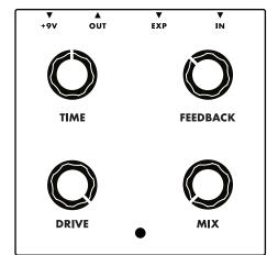
**DRIVE -** A pre-delay circuit that provides greater than 22dB of gain to both input and delayed signal. At low ranges it is excellent for creating subtle boost and mild tonal coloration. At middle position the sound becomes more mid-forward and punchy. At its maximum position, you have an incredibly natural boost/overdrive in your delay pedal that is great by itself or paired with the MF Drive.
