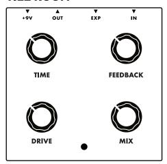
MIX -Allows you to determine the blend between dry and effected signals. At minimum, delay trails are nearly inaudible. This is useful for ghost delays, and creating natural room-verb sounds. At maximum, your dry signal is removed completely, which allows the MF Delay to work perfectly in an amplifier effects loop.
