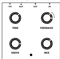
TIME - Adjustable from 35mS - 700mS. At shorter settings, delay repeats are brighter and more articulate - perfect for slap-back and plate-style reverb/delay. As you increase the Time, the delay trails become warmer causing sounds to move and decay naturally under each new note or chord.
