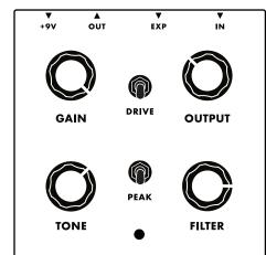
**TONE -** A variable Lowpass/Mid-Scoop/Highpass voicing section sent through a boutique FET for color. At minimum, the sound is dark and full. Approaching the Mid position the sound varies from a slightly scooped American tube amp to a more British, mid-forward tone. At maximum position, the sound is present and articulate with a smooth, rolled of low-end.
