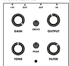
**OUTPUT -** The output level of the MF-DRIVE is extremely hot to offer a wide range of tones from clean to dirty. With proper gain-staging, the MF Drive can also be used as a boost or wah pedal.
