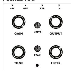
**GAIN -** Sets the input level sent through the OTA before passing through the 4-pole Moog Ladder filter. At lower settings, the MF Drive is cleaner with a smooth breakup. As Gain increases, OTA and filter distortion increase causing the MF Drive to become more aggressive and reactive to picking dynamics.
