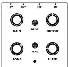
FILTER - Interacts heavily with the Tone knob and filter Peak switch. With Peak off, the filter can be used to reduce top end and add heft to an amplifier. With Peak engaged, the filter can be used to add low, mid, or high frequency boost to your instrument. The MF-Drive by nature has a large bottom end, so this position is extremely useful for dialing in a more focused tone.
