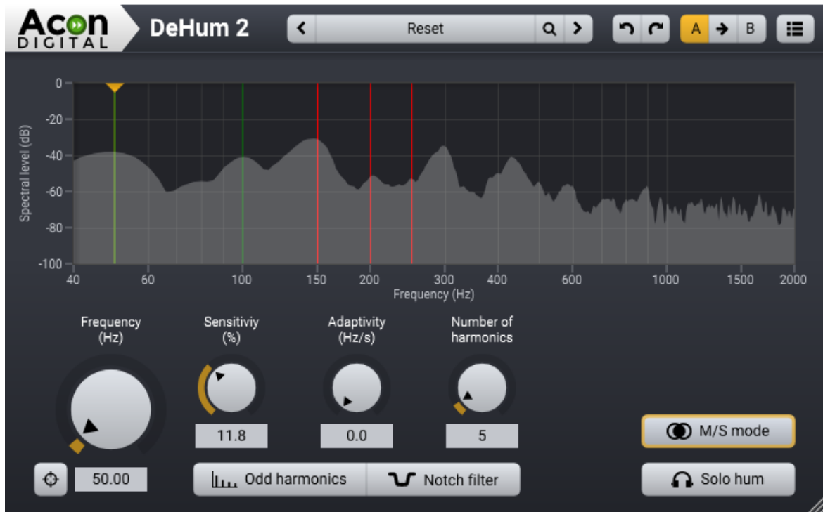
The DeHum 2 user interface with green and red lines indicating the hum harmonics. The lines turn green when hum is detected.
