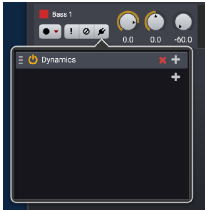
The track insert editor where you can add and remove track processors.
