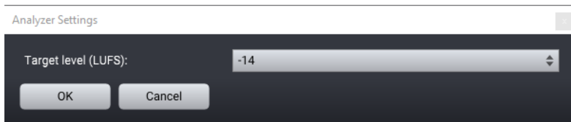
The Loudness Meter Settings lets you select the target level in LUFS
