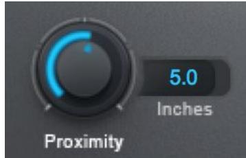
Proximity effect is a boost in bass frequencies that results from placing a directional mic close to a sound source.
