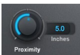
*Proximity effect is a boost in bass frequencies that results from placing a directional mic close to a sound source.*
