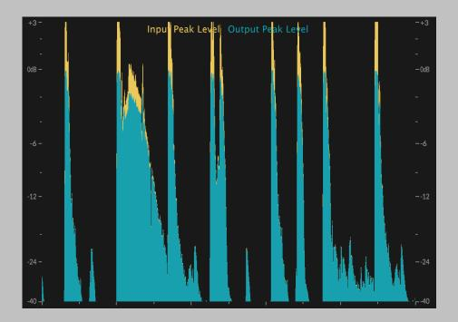
The WAVEFORM DISPLAY sits below the parameters section when the WAVEFORM button is selected, and shows how the Saturate algorithm clips the incoming audio. The input audio waveform (scaled by the desired gain) is shown in yellow with the output audio waveform in blue on top of it. This way, when the output is lower than the gained up input you can see the yellow peak out from behind the blue. This allows to to see how the Saturate algorithm is effecting your audio.
