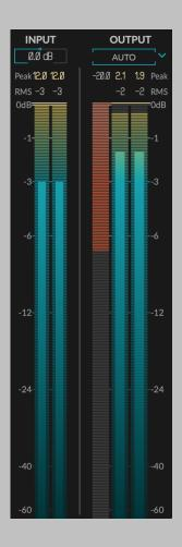
The left and right hand sides of the plug-in have matching vertical bar meters which display the INPUT (on the left) and OUTPUT (on the right) levels in levels in Peak (horizontal ticks), RMS (solid bar and numerical display), and Peak Hold (numerical display) formats. These meters are always present in the display and clicking the Peak Hold section, or bypassing the plug-in will clear the held peak value.
