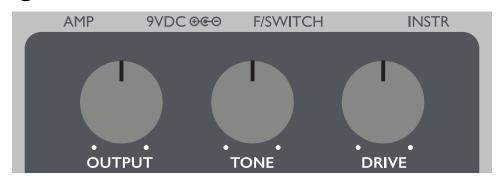
**9VDC:** Connect a 9VDC 2.1mm centre-negative mains power adaptor (minimum 100mA).
