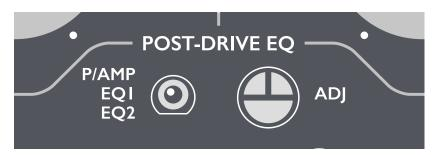
The **POST-DRIVE EQ** ensures compatibility with a wide range of amplifiers. Instead of altering your amp or its tone controls to suit the DELUXE61, set your amp for the desired clean sound then use the EQ controls to tailor the pedal's output accordingly.
