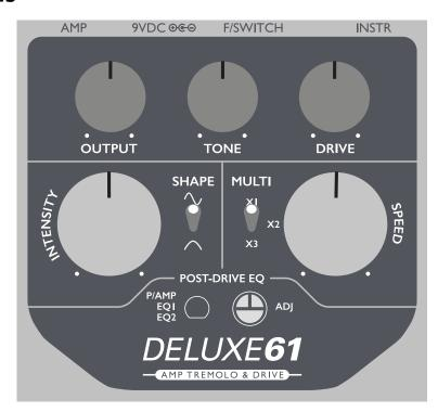
**ON (footswitch):** Turns the pedal on and off. When the pedal is engaged, the LED will illuminate. When the tremolo is active, the LED will flash green (at the tremolo speed). When the tremolo is bypassed, the LED will light up red. Please note: as the tremolo is part of the emulated amp circuitry, it cannot be activated independently.
