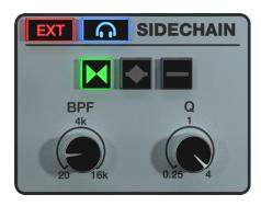
The sidechain section determines what audio will be used to send to the threshold detector. Use this to dial in with more detail how you want Big Beautiful Door to react to the incoming audio level.
