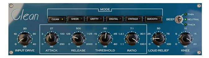
**Drive** - This knob controls the input gain to the plugin. It also provides analog saturation as you increase the gain. No saturation will be applied when the drive is on 0dB.
