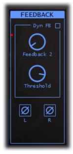
**Feedback** - This knob controls how much of the output of the delay is fed back into it's input. Note that there is a limiter built into the feedback loop, which allows you to get insane feedback without blowing out your speakers. It also makes for some fun effects.
