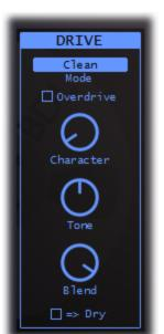
**Drive** - This knob controls how much distortion is applied to the input of the delay. Disabling the drive sends a clean signal to the delay section.
