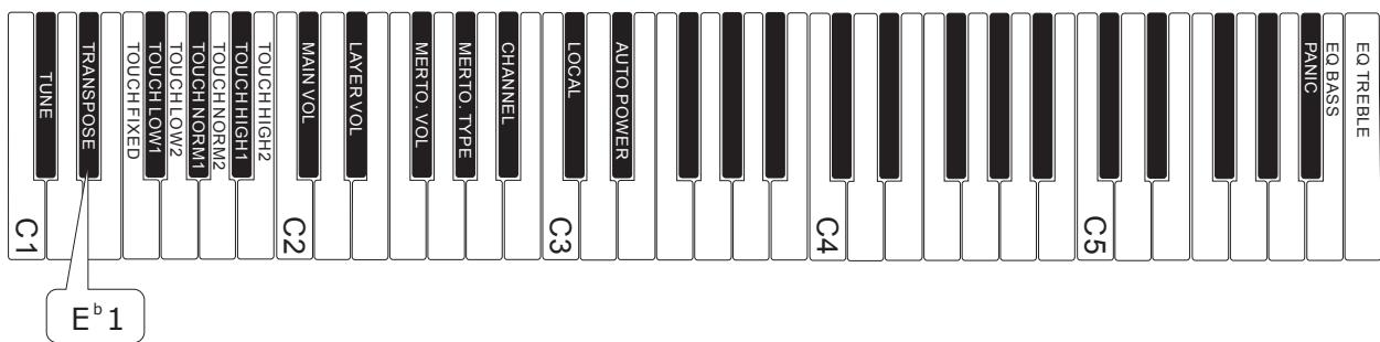
Piano key C3 represents the default standard tuning, and the keys an octave above and below C3 can be used to select the desired key signature. For example, pressing key B2 would transpose down one semitone, whereas pressing key C#3 would transpose up one semitone.
