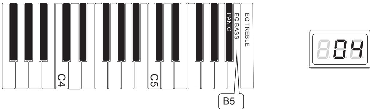
The bass EQ can now be changed by pressing the white keys from A1 (-12dB) up to D5 (+12dB.) The bass level will be shown on the display.
