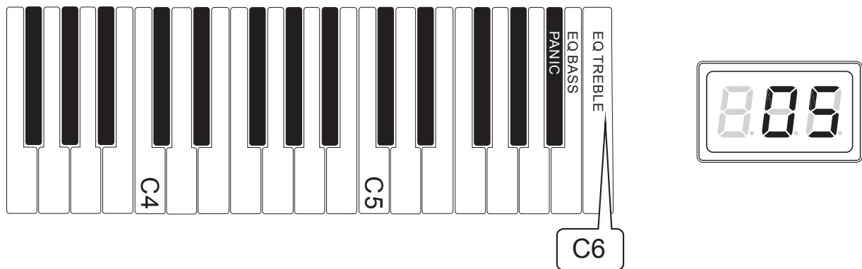
The treble EQ can now be changed by pressing the white keys from A1 (-12dB) up to D5 (+12dB.) The bass level will be shown on the display.
