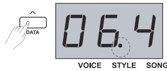
**Please Note:** Always use three digits when using the assigned key(s) to select the desired data value. For example, press and hold the [SHIFT] button, then tap 0,6,4 in sequence to set the data value 64.
