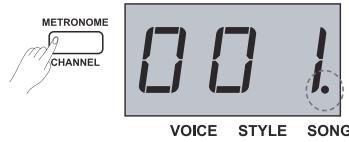
**Please Note:** Always use two digits when using the assigned key(s) to select the desired command value. For example, press and hold the [SHIFT] button, then tap 0,1 in sequence to set the channel value 01.
