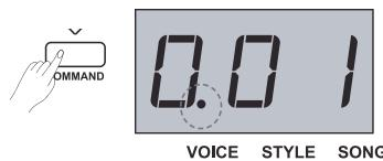
**Please Note:** Always use three digits when using the assigned key(s) to select the desired command value. For example, press and hold the [SHIFT] button, then tap 0,6,4 in sequence to set the command value 64.
