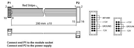
Connect end P1 to the module socket
