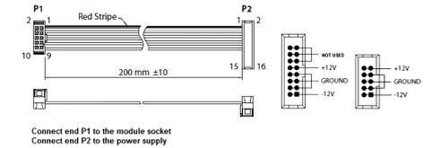
Connect end P1 to the module socket
