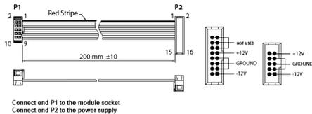
The 911 comes with the required power cable for connecting to a standard Eurorack power supply system. Follow these steps to connect power to the module. It is easier to make these connections before the module has been mounted into a rack case.
