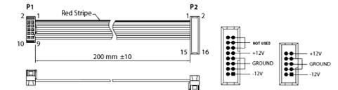
Connect end P1 to the module socket
