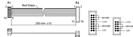
Connect end P1 to the module socket
