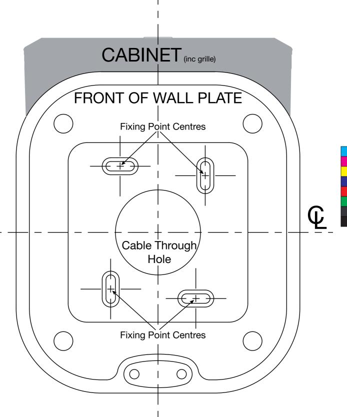
This template shows the fixing points to secure the Apex 10 to a ceiling.
