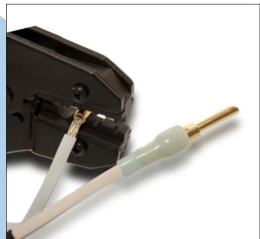
All factory crimping is performed using dedicated machine tools. The picture illustrates the process using a hand crimping tool.
