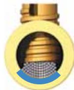
Cross section of standard screw lock termination.
