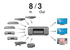
For connection to a broad range of digital sources, this unit features 8 HDMI inputs, including 1 on the front panel that lets you quickly and conveniently connect a camcorder, game console or other HDMI-equipped device. There are dual HDMI outputs for the main room, and a third HDMI output for ZONE2.
