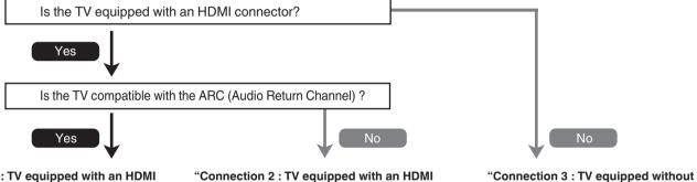
"Connection 1 : TV equipped with an HDMI connector and compatible with the ARC (Audio Return Channel)" ((F) p. 74)
