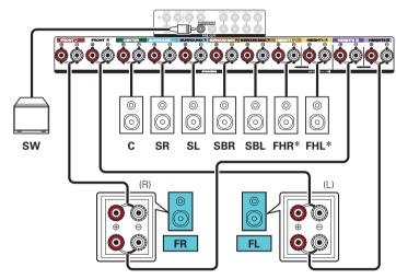
\* The height speakers, ceiling speakers and Dolby Atmos Enabled speakers can be connected to the HEIGHT1 speaker terminals. Set the speaker to be connected from "Height" - "Layout" in the menu. (127 p. 223)
