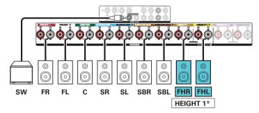
\* The rear height speakers can be connected instead of the front height speakers. In this case, set the height speakers to be connected under "Height" - "Layout" in the menu. (27 p. 223)
