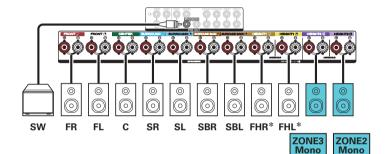
\* The height speakers, ceiling speakers and Dolby Atmos Enabled speakers can be connected to the HEIGHT1 speaker terminals. Set the speaker to be connected from "Height" - "Layout" in the menu. (12 p. 223)
