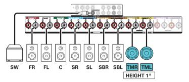
\* The top front or top rear speakers can be connected instead of the top middle speakers. In this case, set the ceiling speakers to be connected under "Height" - "Layout" in the menu. (\*\*\*) 2.23)
