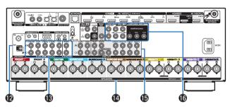
P FM/AM antenna terminals (ANTENNA)
