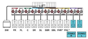
\* The height speakers, ceiling speakers and Dolby Atmos Enabled speakers can be connected to the HEIGHT1 speaker terminals. Set the speaker to be connected from "Height" - "Layout" in the menu. (Pp. p. 223)
