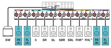
\* The height speakers, ceiling speakers and Dolby Atmos Enabled speakers can be connected to the HEIGHT1 speaker terminals. Set the speaker to be connected from "Height" - "Layout" in the menu. (127 p. 223)
