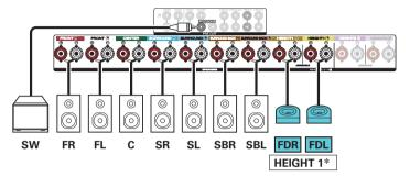
\* The surround Dolby speakers can be connected instead of the front Dolby speakers. In this case, set the Dolby Atmos Enabled speakers to be connected under "Height" - "Layout" in the menu. ( \*\* p. 223)
