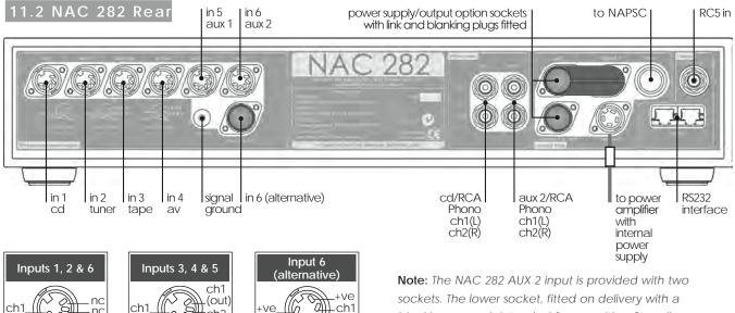
sockets. The lower socket, fitted on delivery with a blanking cover, is intended for use with a Stageline or Prefix Phono stage and incorporates an appropriate DC power supply. The two sockets must not be used simultaneously.
