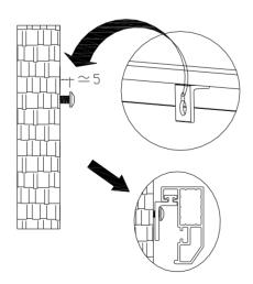
E: Mount the screen. Slide the mounting brackets until they line up precisely with the screws. Lift the frame onto the screws. The screws need to be inserted into the mounting brackets.
