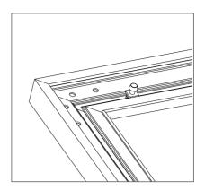
8. Screw in 4 corner screws into each corner of the frame, but do not tighten until all corners have been accurately aligned. Once all corners are accurately aligned tighten the screws.
