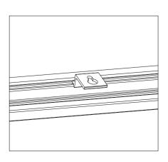
7. Slide the metal corner pieces into the ends of the long frame rails. Now put all frame pieces together forming the assembled frame.
