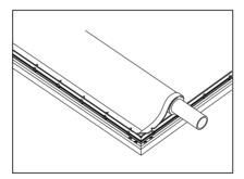
10. Insert the rods into the pockets on the edges of the screen, using the appropriate rods for each side.
