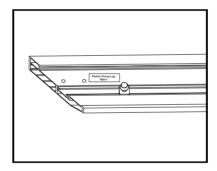
6. Slide the mounting brackets into place. There will be four mounting brackets. Two go on the top rail and two go on the bottom rail.
