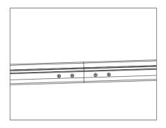
5. Slide plastic snap lugs into the frame rails, see stickers on each frame rail for the required quantities.
