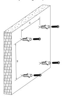
D: Leave about 1/4" (5 mm) of screw thread exposed.
