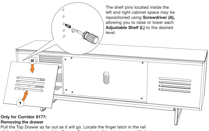
Pull the Top Drawer as far out as it will go. Locate the finger latch in the rail of the slide on each side of the Drawer. Press the Left Latch down and lift the Right Latch up simultaneously and slide the Top Drawer the rest of the way out. (Be careful of grease residue on drawer slides)
