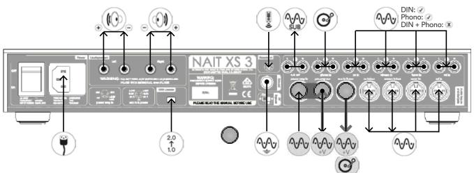
Note: The link plug should be removed only if a power supply upgrade is to be used, an alternative preamplifier is to use the NAIT XS 3 power amplifier section, or an alternative power amplifier is to use the NAIT XS 3 preamplifier section. It should remain fitted in all other circumstances.
