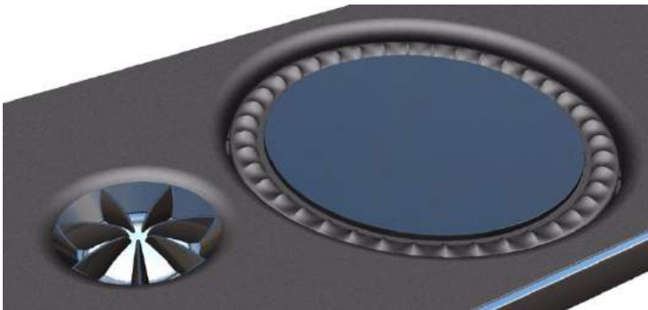
• FEA model showing the Z-Flex surround deformation as the cone moves forward.
