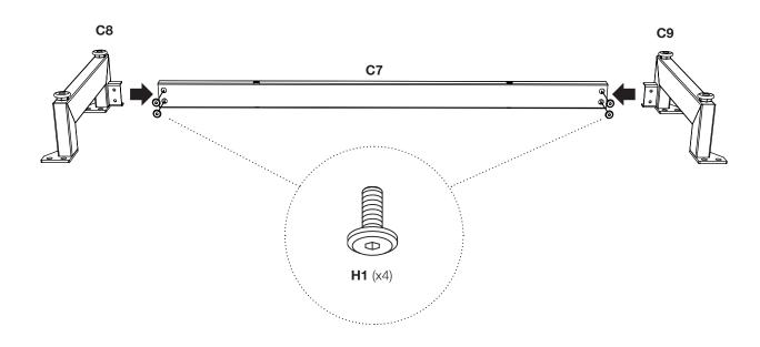
Step 3 - Attach Base Assembly to Cabinet using Screws H1 and H3 and tighten with Hex Wrench.
