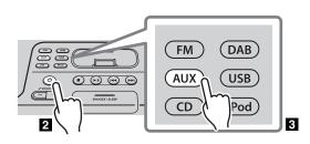
Using a commercially available 3.5 mm miniplug cable, connect your external device to the AUX on the rear panel of this unit.
