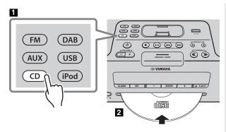
■ Press the CD source button to switch the audio source to CD.
