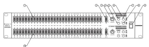
(1) Equalizer level sliders - Independent Equalizer sliders are provided for each frequency area (The S curve 231 provides 31 frequency areas).Calibration markings on either side of each Equalizer slider allow you to cut or boost each frequency area. As described below, the exact action of the Equalizer sliders depends upon the setting of the Range switch as well as the setting of the Cut Only switch (see #3 and #5).
