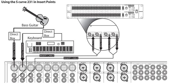
You can use the S curve 231 in your mixer's insert points if you want to equalize two mono channels individually in the mix. In this example the S curve 231's Channel 1 INPUT and OUTPUT are inserted on a bass guitar channel using a 1/4-inch TRS to 2 x 1/4-inch TS "Y" cable, and the Channel 2 INPUT and OUTPUT are inserted on a keyboard channel using the same type of cable. For more information on cable wiring see the S curve 231 Wiring Guide page 15 in this manual.
