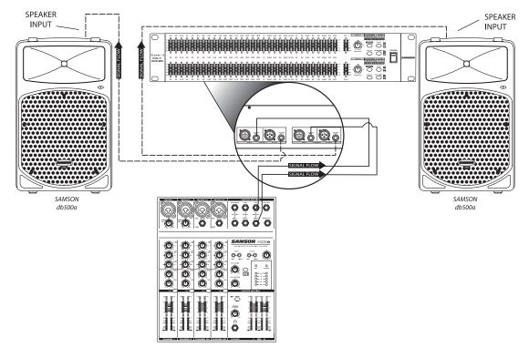
In this example, the mixer's stereo output is connected to the S curve 231's inputs. Then, the S curve 231's outputs are connected to the inputs of each active (self-powered) loudspeaker.
