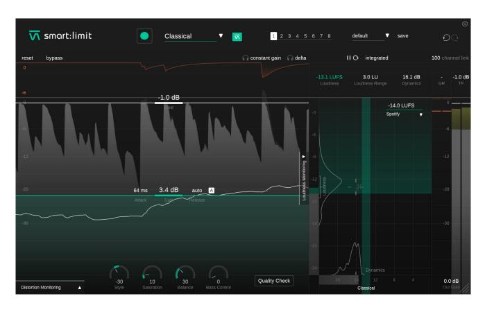
smart:limit provides a unique instant impact prediction feature for an optimized workflow. While loudness monitoring tools typically require you to restart the loudness measurement from scratch after changing parameters, smart:limit's loudness metering (Loudness Meter, Dynamics Meter, readouts and histograms) reflects every parameter change in real-time without having to repeatedly playback the entire input signal.
