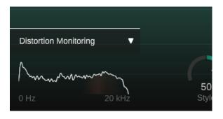
Click on the arrow in the lower left corner to expand the Distortion Monitoring display. The spectral representation indicates the amount of distortion in bright red for different frequency regions.
