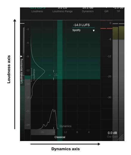
When using a limiter, the loudness and the dynamics of a track are highly interconnected. Increasing the input gain increases the loudness of the signal, but also reduces the dynamics as soon as the signal hits the limit. The Loudness and Dynamics Grid helps to find the right trade-off between the current loudness of a track and its dynamics.
