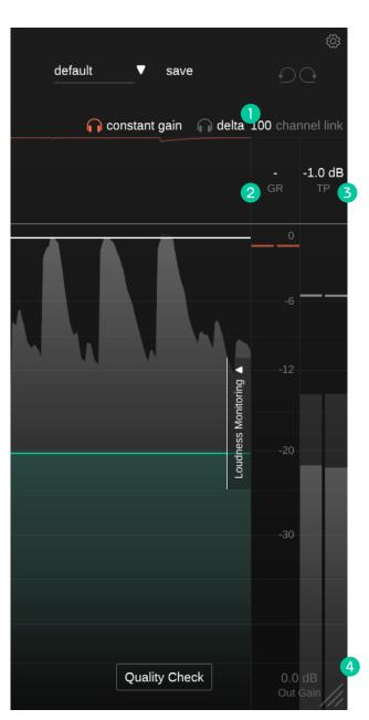
For quick monitoring, smart:limit provides a classical gain reduction meter and a true peak output meter on the right-hand side of the interface. Expand the Loudness Monitoring section for extensive insights into the loudness and dynamics of your track (see page 13)
