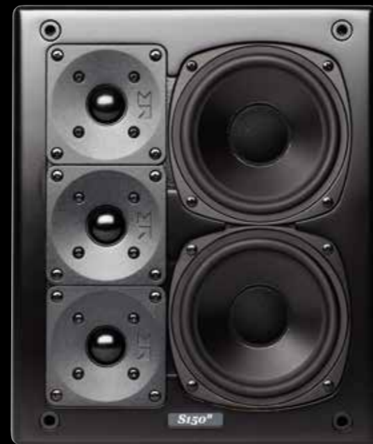
Placing the drivers side by side in close proximity reduces cabinet size significantly for enhanced structural integrity at no sacrifice in performance. Because all drivers are close to the edge of the baffle, diffraction phenomena are virtually eliminated.
