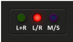
**L+R:** When activated, the left and right channels are linked. This allows for the edge reduction in the target area to be the same for both channels.
