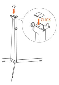
4. Apply the click-on stainless-steel cover plate  $\mathbb{P}$  on top of the steel bracket  $\mathbb{O}$ .
