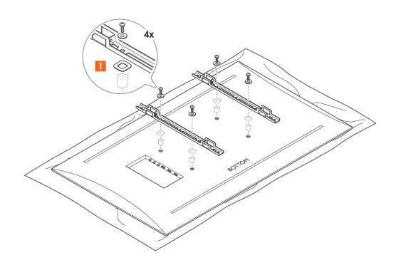
1. Fix the protective TV patches () onto the interface strips ().
