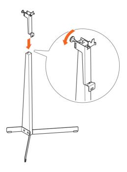
3. Slide the **steel bracket** (1) over the top of the **wooden stand** (R). Use the knob (see illustration) to fasten the **steel bracket** (1) to the top of the **wooden stand** (R).
