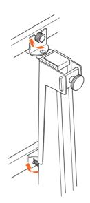
2. When the TV is mounted, secure the **interface bars** (B) to the **steel bracket** (U) by fastening the **thumb nuts** (N).
