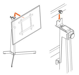
Carefully lift the TV and lower the upper interface bar
