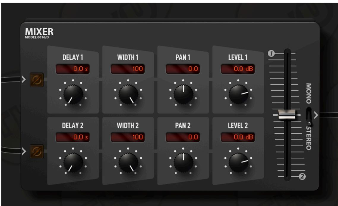
**PAN:** sets the panpot or panorama position of the input channel at the output. For stereo signal it acts as a
