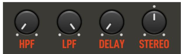
**HPF:** a High Pass Filter, used to attenuate the low frequency harmonics.
