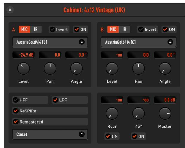
**A & B** are the sections which control the two main microphones. If you click on **IR**, instead of using a microphone you can load an IR. When **MIC** is selected, you can choose a microphone from a list of 18.
