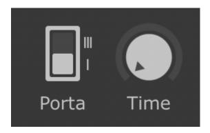
If a note is playing (ie, the MIDI note has not ended and the envelope has not reached its Release phase) and another note plays, the AX73 Portamento effect causes the pitch to bend from the first note to the second. The length of this glide is determined by the **Time** dial.
