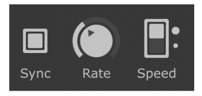
The **Speed** knob can be set to Slow or Fast. When the **Sync** button is active, this knob does not do anything. However, when **Sync** is not active, the **Speed** knob changes the available range frequencies that the LFO can be set to oscillate to with the **Rate** dial.
