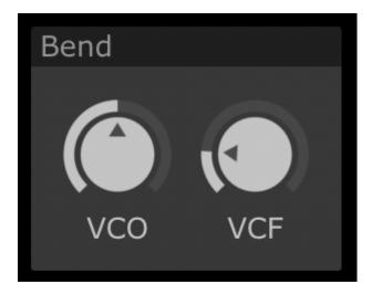
Your pitch wheel can also control the cutoff of the filter with the **VCF** dial. You can set both pitch and cutoff to be modulated by the wheel, by differing amounts, or just choose one of these.
