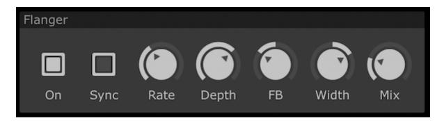
Control the depth of the flanger with the **Depth** dial, the Feedback with the **FB** dial, the stereo image of the flanger with the **Width** dial and the dry/wet mix with the **Mix** knob.
