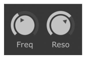
The filter is capable of self-oscillation when the Resonance is set high enough.
