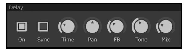
The **Pan** button introduces ping pong delay. Turning the dial right will pan the first tap right, turning the dial left will pan the first tap left. The more you turn this dial left or right, the more both left/right delays will be spread out to their side of the stereo image.
