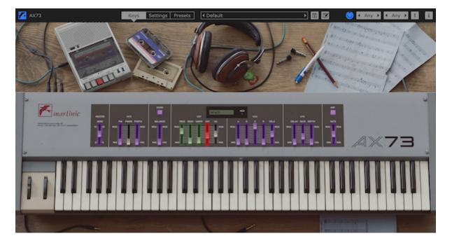
Controls that can be learned will turn **purple**. Click a control in order to start assigning it, and the control will turn **red**. Next, move the knob, fader or other control that you want to assign to this parameter on your real-life MIDI keyboard. The keyboard should now assume control over the parameter, and the control will turn **green** to indicate that it has been assigned.
