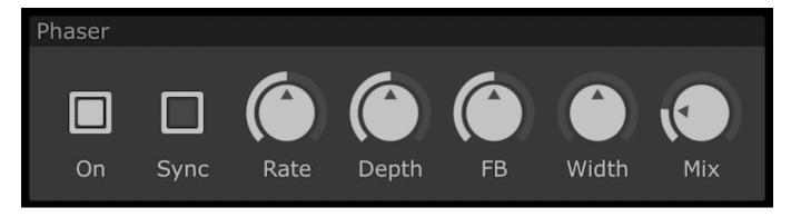
The depth of the phaser is controlled by the **Depth** dial, **FB** controls the level of feedback, **Width** the stereo image of the sound and **Mix** the dry/wet balance.
