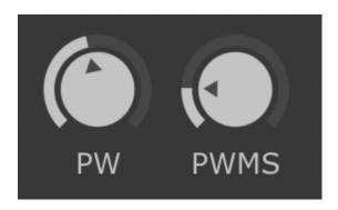
The PWMS modulation source comes from one of the LFOs, and is actually an alias for that LFO's Rate control. In the default patch, LFO 4 has PWM set as its destination, but any LFO can be set to modulate PW. If multiple LFOs target PWM, then it will use the LFO with the highest number (ie, if both LFO 1 and 4 target PWM, then it will use LFO 4).
