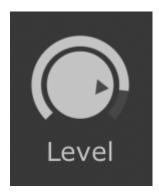
The VCA Level control can be particularly helpful to compensate for the saturation introduced by the Filter stage of the synth. The filter can increase the level of sound (when using added resonance) or reduce it (when filtering heavily), so the Level control in this section can help to bring the signal back to a steady level.
