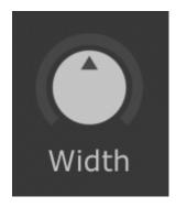
If Keyboard Assign is set to Dual or Unison, then **Width** controls the stereo spread of the voices within a single note. In this mode there's no difference between lower or higher keys, they're all the same.
