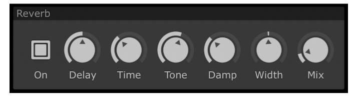
The **Damp** dial fades out high frequencies more quickly than low frequencies, to greater or smaller extents. The **Width** knob alters the stereo image of the reverb (with values below 50 reversing the channels) and the **Mix** dial dictates the dry/wet balance.
