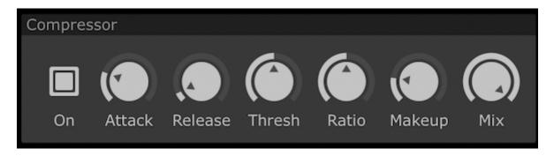
The **Threshold** knob determines the minimum volume at which the compressor begins to take effect.
