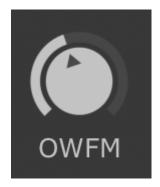
Because this is an audio-rate modulation routing, the behaviour of this function is dependent on the filter's cutoff and the notes played – the effect will often be different for lower notes than it is for higher ones.
