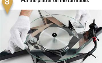
The turntable should always be placed on Put the platter on the turntable. a flat surface. Check with a spirit level\*.
