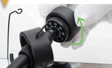
Put the loop of the Anti Skating Weight (a) in the outer notch on the tonearm post.
