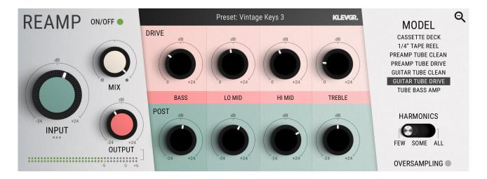
The seven models available are based on real analog gear individually measured in two dimensions; gain responses (-inf dB to +6 dB) at the frequency spectrum 20Hz to 20kHz. This data is used to transform input audio to output audio.
