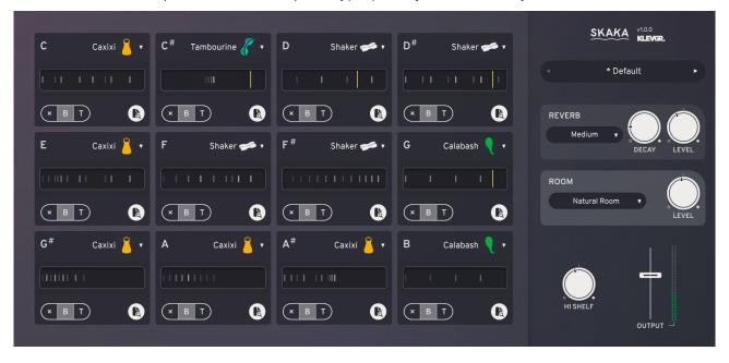
All continuous parameters (knobs and sliders) in this plug-in are automatable with an exception for events in the sequencer and the parameters inside the Humanize settings editor.
