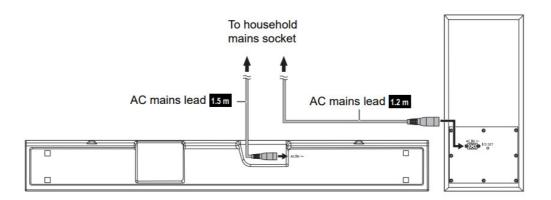
Note: The active subwoofer is in standby condition when the AC mains lead is connected. The primary circuit is always live" as long as the AC mains lead is connected to an electrical outlet.
