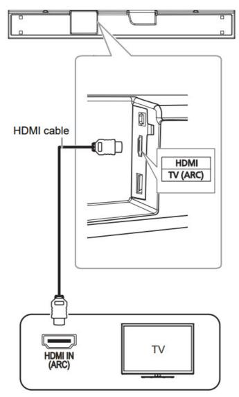
ARC (Audio Return Channel) ARC is an HDMI function that lets you enjoy both sound and TV pictures with one HDMI cable, the optical digital audio cable that is usually required in order to listen to sound from a TV is no longer required.
