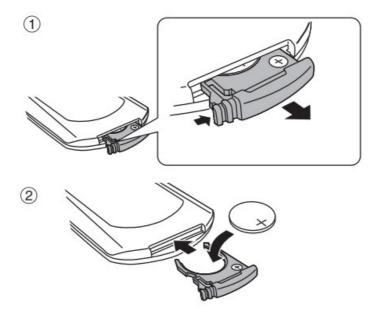
Insert a new battery with the (+) side facing up.
