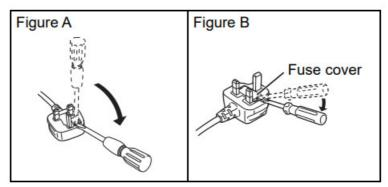
2. Replace the fuse and close or attach the fuse cover.
