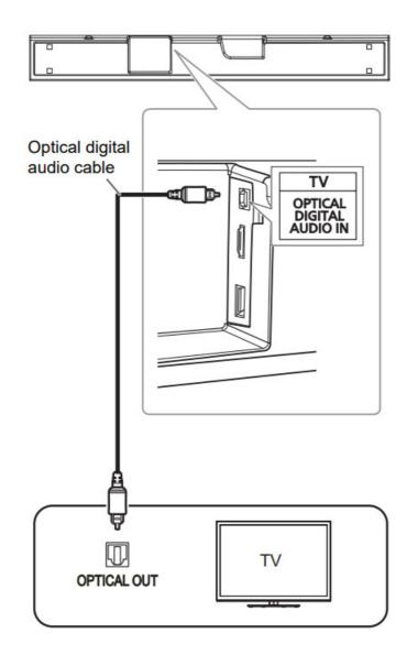
When connecting the optical digital audio cable, observe the orientation and insert the tip correctly into the terminal.
