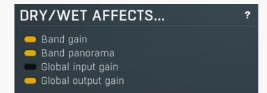
Dry/wet affects... panel controls which multiband parameters are affected by the global dry/wet controls. Dry/wet generally controls the mix between the processed and input signal, however it is often advantageous to support its function with other parameter. In most cases it is good to enable everything except for global input gain. However note that this 'default' is not specified for most plugins for sake of maintaining backwards compatibility.
