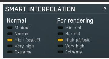
Smart interpolation panel controls the depth of the smart interpolation algorithm, which controls the parameters in order to provide maximum audio quality and lower the chance of zipper noise. Smart interpolation is engaged whenever you change any parameter via the GUI, modulators, multiparameters, MIDI or automation.
