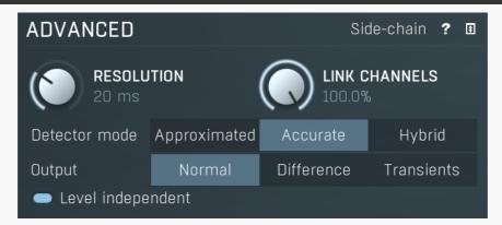
Advanced panel contains more advanced transient processor parameters.
