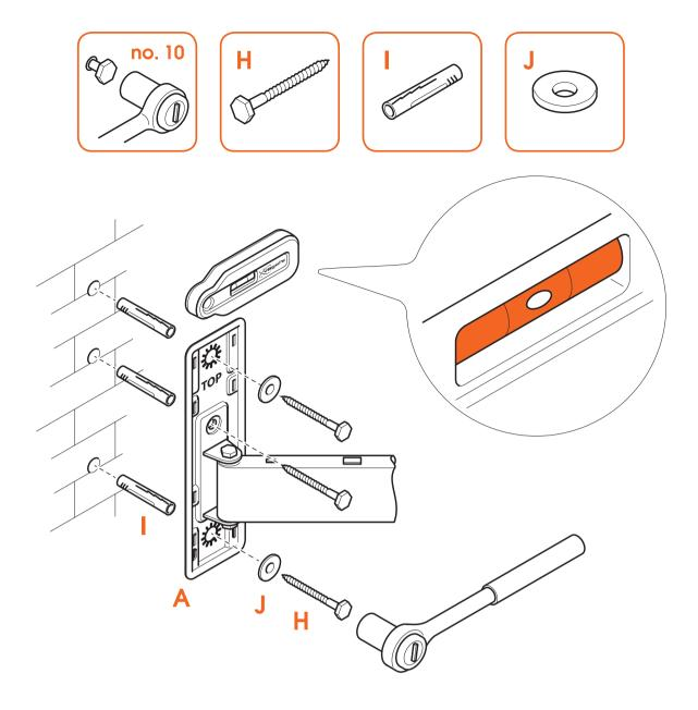
3. Attach the wall mount (A) to the wall with the screws (H), washers (J) and plugs (I). Use the spirit level to level the wall mount.
