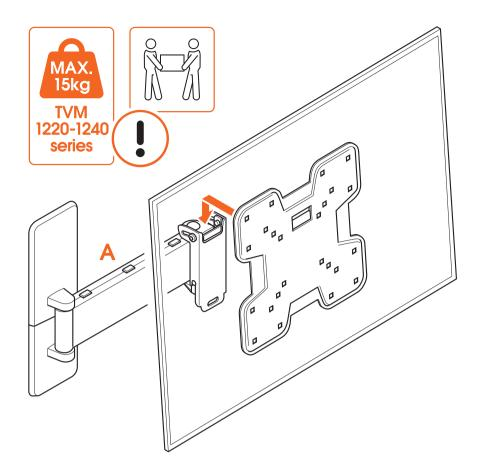
1. Carefully lift and attach the TV to the wall mount (A).
