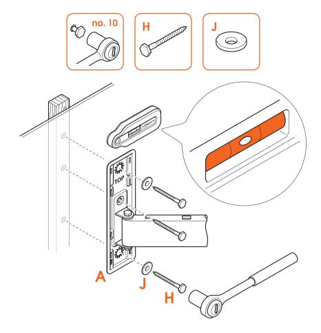
4. Attach the wall mount (A) to the wooden wall with the screws (H) and washers (J). Use the spirit level to level the wall mount.
