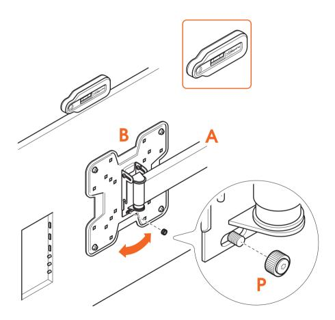
2. Attach the adapter B to the wall mount A with the thumbnut P. Make sure the TV is levelled, using the spirit level.
