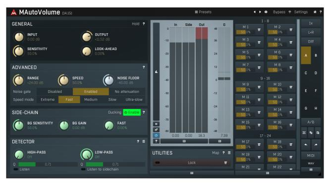
MAutoVolume is a solution to a common problem - stabilizing loudness of a front instrument, such as a vocal, a bass or a saxophone. Although you can use a compressor for this, setting it up may be very time consuming and the results questionable. You can also manually automate the volume fader, which is the method most engineers used so far, and it is not exactly ideal as well. MAutoVolume solves this problem quickly, easily and with astonishing results.
