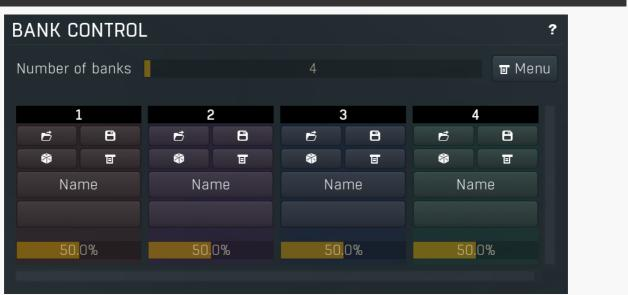
Bank control panel is available only in **Banks mode** and contains tools to define the banks between which the multiparameter is interpolating. The multiparameter stores parameter values for each bank. Here you can load and save these values.
