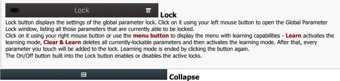
Collapse button minimizes or enlarges the panel to release space for other editors.
