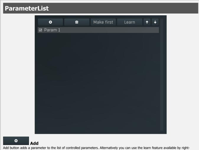
Add button adds a parameter to the list of controlled parameters. Alternatively you can use the learn feature available by rightclicking the multiparameter button.
