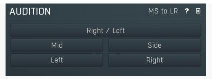
Audition panel contains multiple buttons, which let you audition specific part of the stereo signal. This can be used to understand the stereo field properly and check if the output signal is well ballanced.
