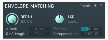
Envelope matching panel lets you automatically match the level envelope in one channel to the other. In most cases one microphone is
