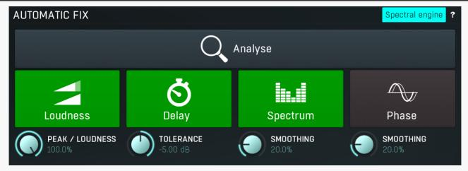
Automatic fix panel contains the core of the plugin - the automatic detection and fixing of various problems. First enable the playback and use the **Analyse** button to analyse your audio. Use the remaining buttons to enable or disable all each of the fixes that the plugin offers to improve the stereo field of your audio material.
