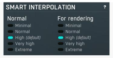
Smart interpolation panel controls the depth of the smart interpolation algorithm, which controls the parameters in order to provide maximum audio quality and lower the chance of zipper noise. Smart interpolation is engaged whenever you change any parameter via the GUI, modulators, multiparameters, MIDI or automation.
