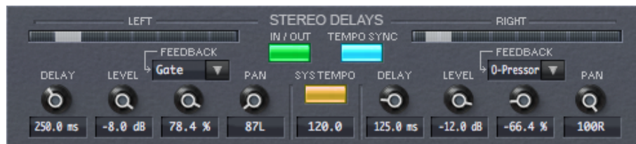
Figure 3.7: UltraChannel Stereo Delays Section
