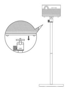
4 Align the threaded hole at the bottom of the machine with the gimbal nut
