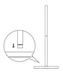
3. Rotate the gimbal clockwise into the connecting rod
