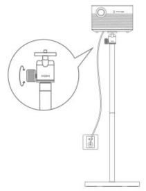
Onnect the power supply, turn on the machine's optical machine and rotate the gimbal knob, project the picture to a suitable
