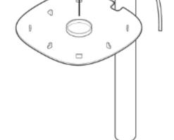
Plug the power cord back into the speaker and place on the top mount, pulling any extra cable down from the top. Tighten the screws and attach the top cap with the notch facing toward the speaker.
