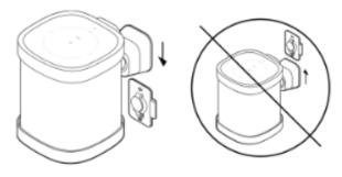
Twist the speaker to position it in place, then turn it right to lock it in securely.
