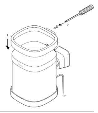
6 Slide the Mount down onto the wall bracket.
