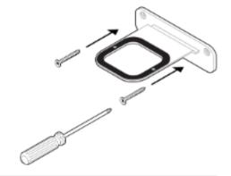
If using wall anchors, use a 5/16" drill bit to drill 2 pilot holes and then insert the wall anchors. Refer to the wall mounting information below for guidelines. Otherwise skip this step.
