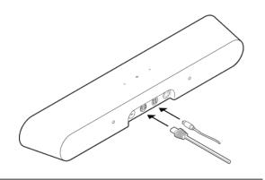
Remove the protective cap, then connect the optical cable to your TV's optical digital OUT port. (The TV's optical adapter's port is "D-
