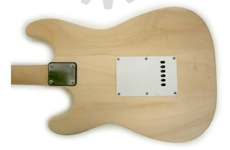
Put the Body (1) and Neck (2) together. Place the Neck Plate (10) with the rubber Pad on the back of the Body (1) in line with the pilot holes, and attach with the 4 x 45mm screw.
